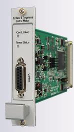
QCM934-200 is a module board with a built-in oscillation and temperature controller
