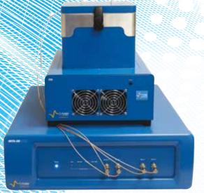
The Intermediate Temperature System (ITS) is a temperature control unit based on **Peltier** effect.
