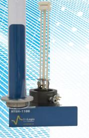
**High Temperature Sample Holder** (HTSH-1100) is a test fixture dedicated to characterization of electrical properties of solid materials using the parallel plate capacitor method over the temperature range between the room temperature and 1100 °C. HTSH-1100 can also be used for heat treatment in controlled atmospheres.
