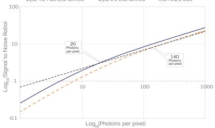
Plot of Signal to Noise Ratio versus Incident Photon Intensity, comparing a back-illuminated EMCCD iXon 888 (13  $\mu$ m pixel size) to 2x2 binned Zyla sCMOS cameras (13  $\mu$ m pixel size after binning)
