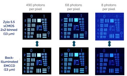
Images at a range of incident light intensity, acquired using backilluminated EMCCD iXon 888 and Zyla 5.5 sCMOS cameras (2x2 binned pixels). At low light intensities, the Signal to Noise Ratio advantage of the EMCCD is apparent (in this example the 8 photons per pixel images).
