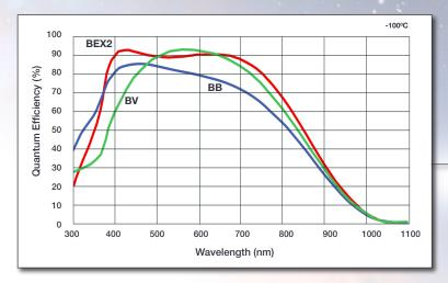
A range of sensor options are available for the iKon-XL 231 that provide high photon collection efficiency for maximizing the SNR. Deep depletion (-DD) sensor options provide extended NIR sensitivity.
